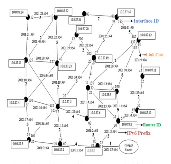
Figure 4.1 Network Topology Discovered by OSPFv3 Based Algorithm
