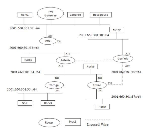
Figure 2.4 The LORIA IPv6 test platform with one LA in each interface of a router [1]
