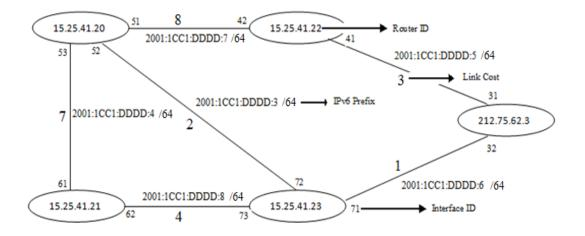
Figure 3.9: Discovered Connectivity Information of an OSPFv3 Area
