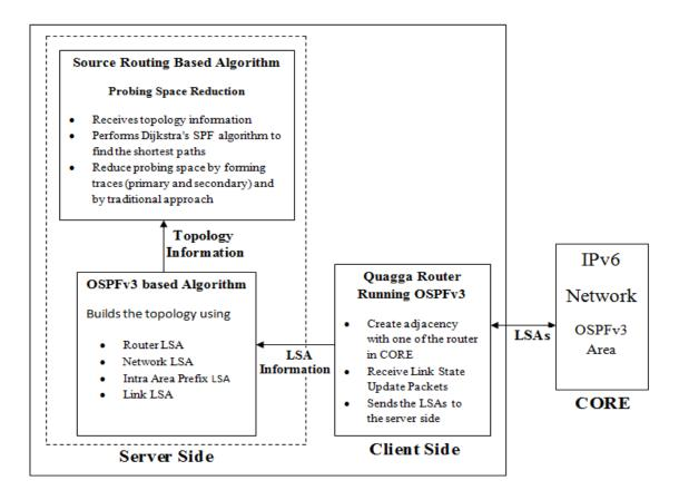
Figure 3.3 Architecture of Topology Discovery and Source Routing based Algorithm
