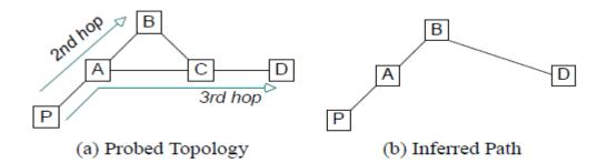
Figure 2.5 Incomplete Discovery Because of Equal Weighted Path [4]
