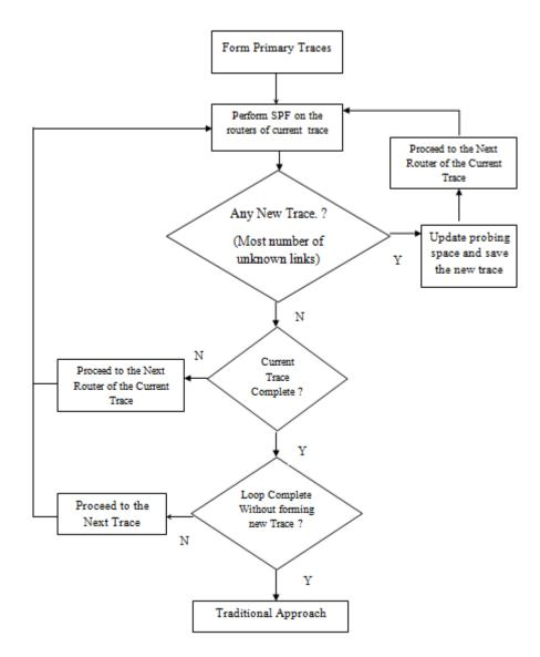
Figure 3.6 Flowchart of Source Routing based Algorithm
