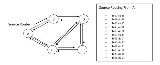
Figure 3.10: Implementation Procedure of Source Routing Based Algorithm
