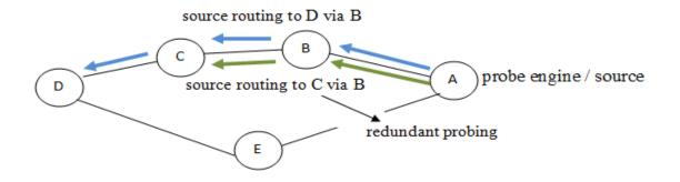
Figure 2.7 Probing Space Reduction in the Same Basic Path
