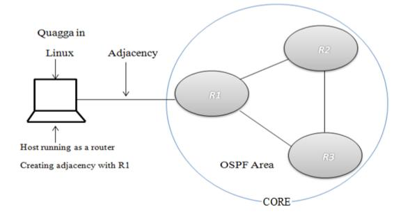
Figure 3.8: Discovering Topology of an OSPF Area
