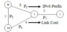
Figure 3.5 Example of the Connectivity Information obtained from OSPFv3
