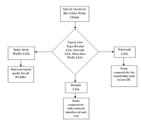
Figure 3.4 Flowchart of OSPFv3 based Topology Discovery Algorithm
