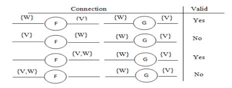
Figure 2.2 Examples of valid and invalid connections between two bridges with different forwarding entries [9]
