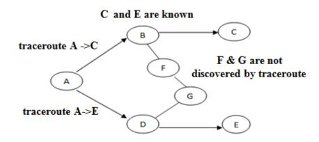
Figure 2.6 Increased Coverage by Source Routing
